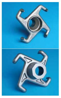
The new single-piece investment casting costs less, is stronger and more dimensionally consistent, more attractive, and includes the Tait logo as cast-in feature. foundry. The company produces net and near-net shapes, ferrous and nonferrous components with assisted design capabilities using computer aided technology. This includes 3-D modeling, as well as solidification simulation.
